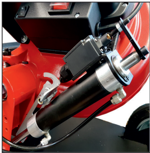
Closed circuit hydraulic system for arm down feed and descent control
